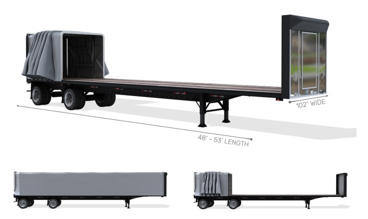
Conestoga semi trailers are designed to offer the enclosed nature of a dry van, while providing the same loading / unloading capabilities of a flatbed. A sliding curtain, when open, allows for freight to be loaded / unloaded from the side, rear, or top. When closed, the curtain offers the weather protection of a dry van without the risk of tarps rubbing against the freight.
