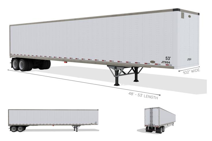
Dry van semi trailers are designed to transport the most versatile of dry products due to the fully enclosed nature of the trailer, which allows freight to be protected from the elements. Palletized products are most common as they can be efficiently and safely loaded / unloaded with a forklift or pallet jack from a dock.
