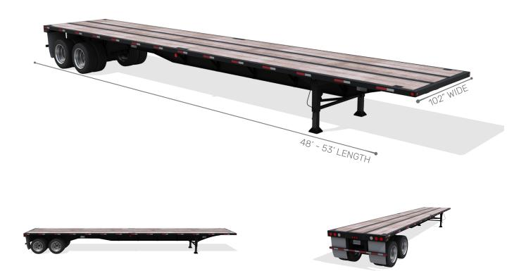
Flatbed semi trailers are designed to transport products which are long, heavy or oddly proportioned which creates a challenge when loading/unloading an enclosed trailer. The open nature of the trailer allows for loading / unloading from the rear, sides or top; allowing forklifts and cranes to create an even lift on the freight. Flatbeds are best suited being loaded / unloaded from the ground, rather than from a dock.
