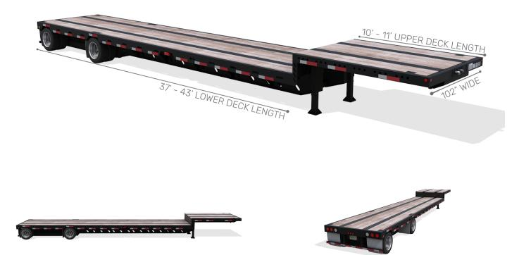
Step deck trailers, also known as drop decks, are designed to transport products which are too tall for a standard flatbed. The trailer consists of two decks, the upper and lower. The use of the lower deck, or well, allows for freight up to 10' high to be legally transported, while still providing the same loading / unloading capabilities of a standard flatbed.
